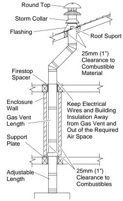
Figure 21 - Typical B-Vent Installation
